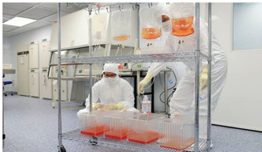
Figure 1: Closed system manufacturing of therapeutic adherent cells in 10-layer vessels using bagged media
